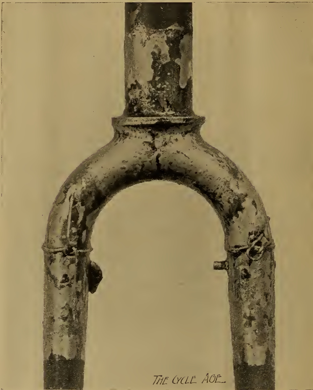
FORK CROWN DIP BRAZED WITHOUT IMMERSING ENTIRE STEM OR BLADES.
